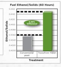
TRANSFERM Yield+ was evaluated against conventional yeast under a high temperature profile in pilot plant scale (7500 gal fermentation) (Figure 4). After 60 hours TRANSFERM Yield+ finished with 2.26% more ethanol than the conventional yeast.
