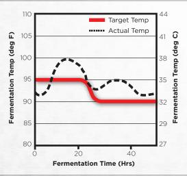
**Figure 2:** Some production facilities may have trouble controlling temperature during hotter months.
