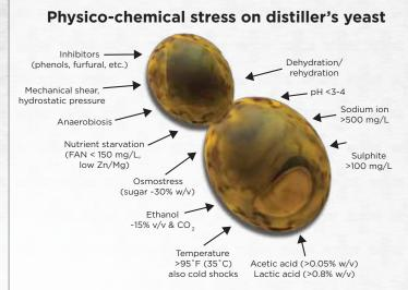
**Figure 1**: Ethanol plant operators must monitor these stress factors through all phases of fermentation or production can be compromised.
