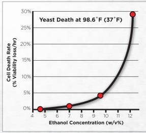
**Figure 3:** Temperature becomes critical in later fermentation stages where ethanol concentration totals are higher.
