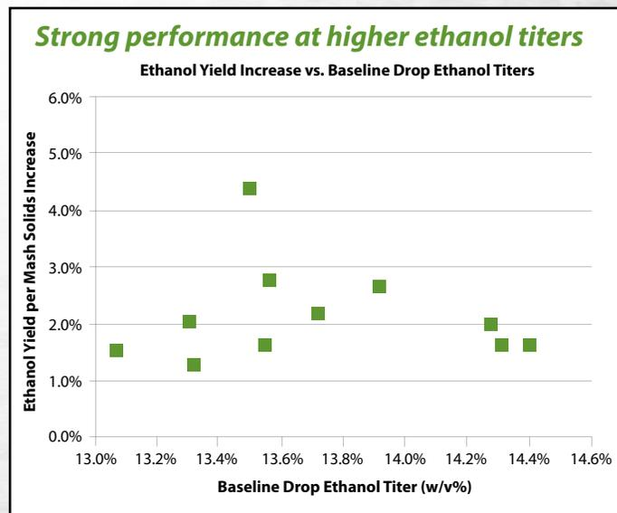
**Figure 2:** Performance of TRANSFERM Yield+ at higher percentage of ethanol titers. Similar performance and correlation to Figure 1 with higher solids. Ethanol yield increased 1-3% with increased ethanol drop titers.
