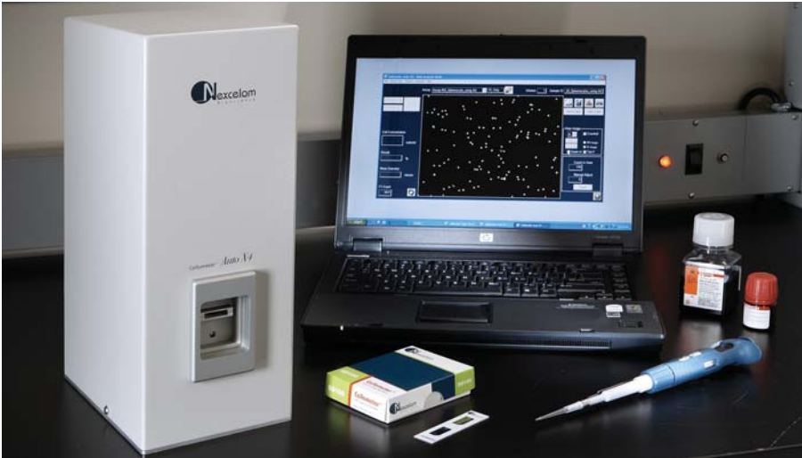
Nexcelom Bioscience's Cellometer allows users to automatically count yeast and view images of the cell sample at the same time.
