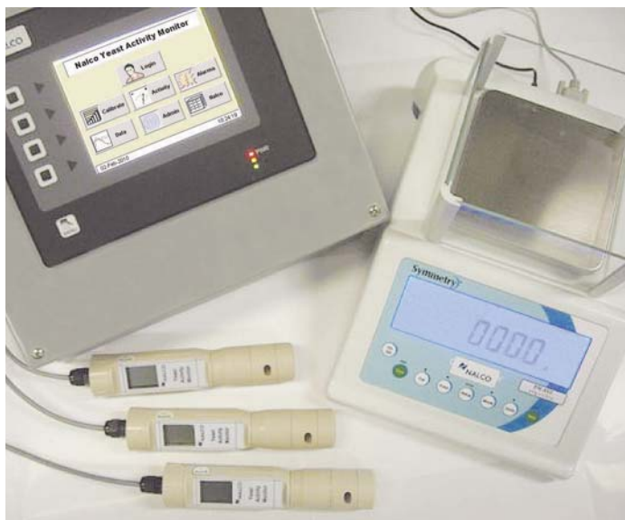
Nalco Co.'s Yeast Activity Monitor measures the metabolic activity of yeast cells.
